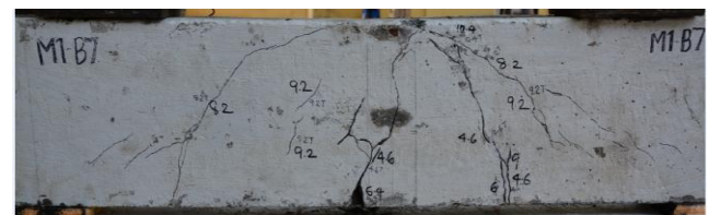
Fig. 10 Typical failure pattern of beam specimen D200
