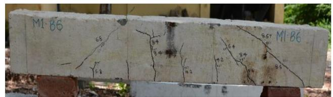
Fig. 9 Typical failure pattern of beam specimen D150
