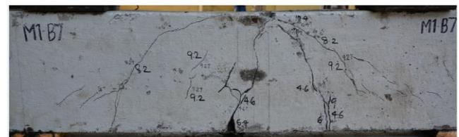
Fig. 10 Typical failure pattern of beam specimen D200
