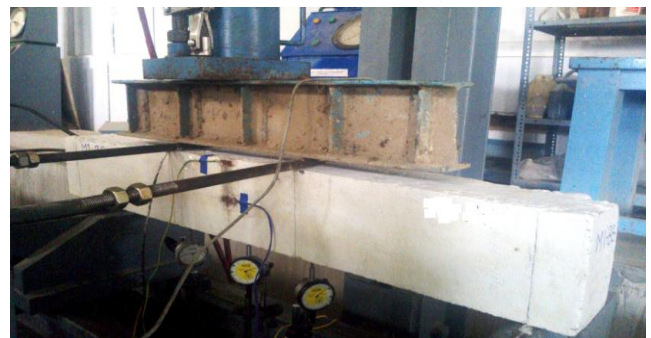
Fig. 2 Typical test setup – Beam specimen with surface strain gauges
