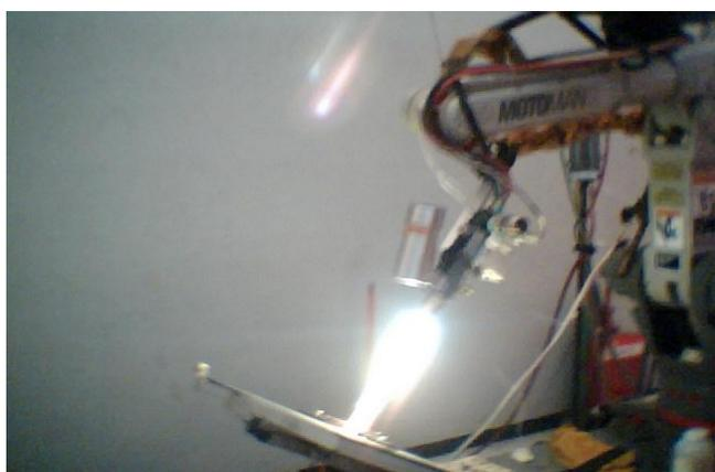
Fig 13: Image of the automated combustion powder thermal spraying process.(ACPTSP) operating.
