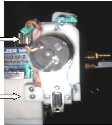
Fig 10: Geared motor coupling to the housing of the automation system.
