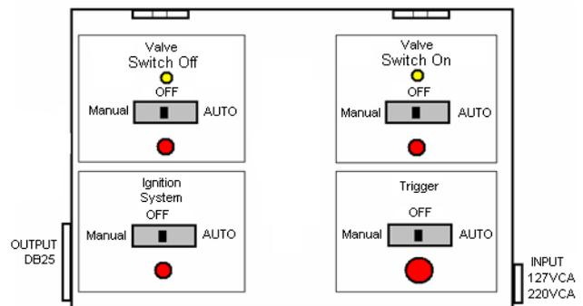
Fig 11: Control Box distribution
