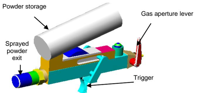
Fig 1: Spray gun, model 5PII, Sulzer Metco.
