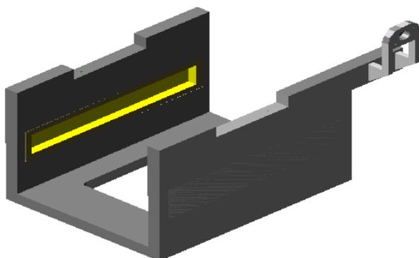
Fig.4: Housing for protection of the trigger.
