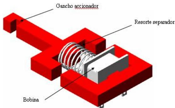
Fig 3: Shutter system for the trigger
