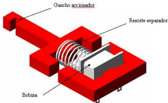
Fig 3: Shutter system for the trigger
