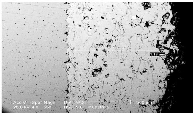
Figure 12. Image of coating of NiCrFeBSi obtained by flame thermal spray on AISI 1018 carbon steel. Thickness of 1.19 mm height of the layer. SEM. BSE
