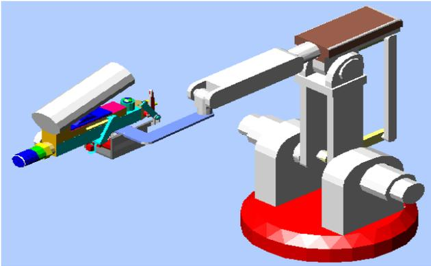
Fig 8: Robot arm with the automated combustion powder thermal spray gun attached.
