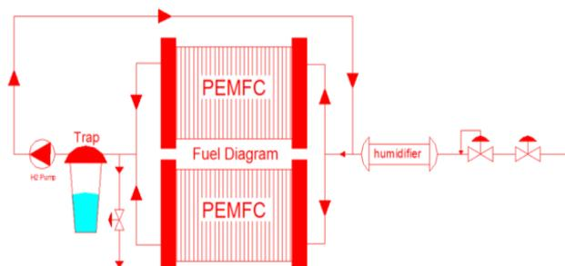
The oxidant circuit of this system is almost similar to its fuel circuit. However, they differ in that the required oxygen is supplied by a compressor which works with dc power and is humidified before entering into the stack. Moreover, the humidifier of hydrogen has been removed in the final test of the system. The humidifier of hydrogen was removed because there was enough humid due to the reaction on the side of anode which was because of the large number of cells.
