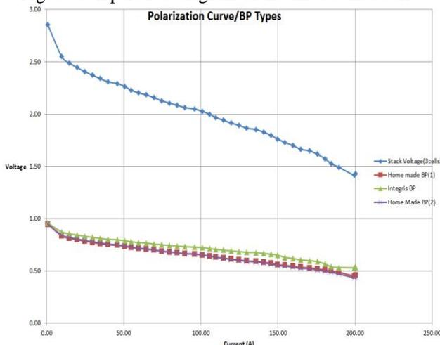
As it is shown in the above diagram, performance of the two prototype samples of homemade production plates and the foreign ones, were so close. After confirming the bipolar samples, producing 130 cells of two 65 cells stacks, which were the main section of the 10kW fuel cell system, were assembled. Then the stages of stack leakage and voltage stability test and MEA break-in test were all performed separately, on each of these two stacks. Then, the two stacks were installed within the system.
