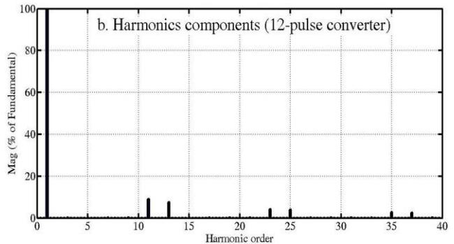
Fig.3 harmonic spectrum of 12- pulse converter
