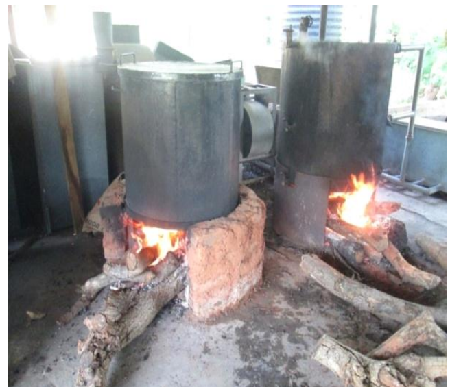
Plate 2. Testing of improved traditional parboiler
