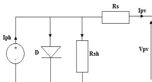
**Figure 1.** Solar PV cell equivalent circuit.
