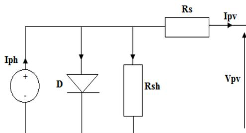
**Figure 1.** Solar PV cell equivalent circuit.
