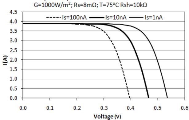
Figure 5. Effects of the diode reverse saturation current on the PV cell output voltage and current.
