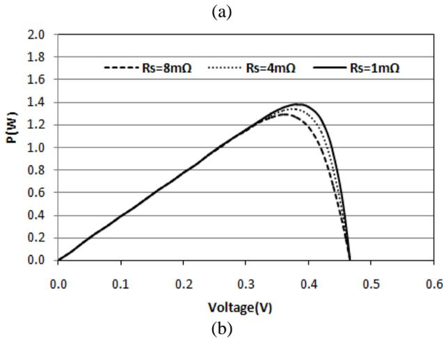
Figure 4. Effects of the series resistance on the current (a) and the power output (b).
