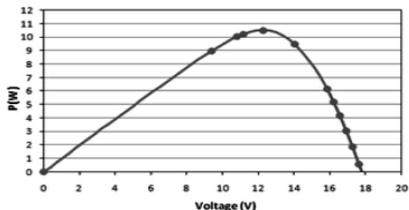
Figure 9. The GE 30 Watt module PV curve. The discrete data points indicate the experimental values
