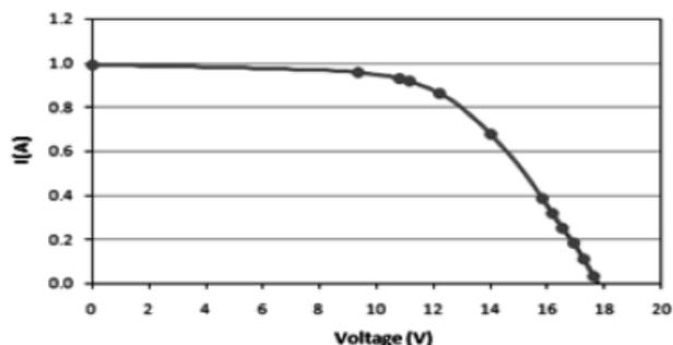
Figure 8. The GE 30 Watt module IV curve. The discrete data points indicate the experimental values
