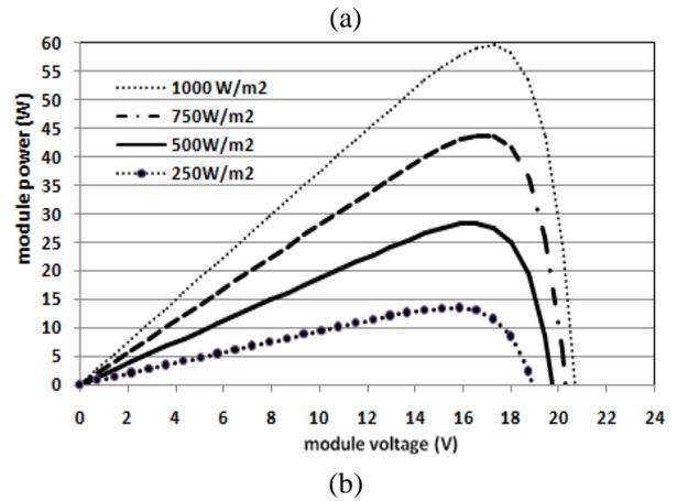
Figure 6. Effects of solar radiation on the current (a) and the power output (b) of Solarex MSX60.
