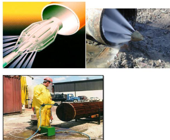
Figure 3: Pipe Cleaning by Jetting (Courtesy: AAA Pipe Cleaning Corporation)
