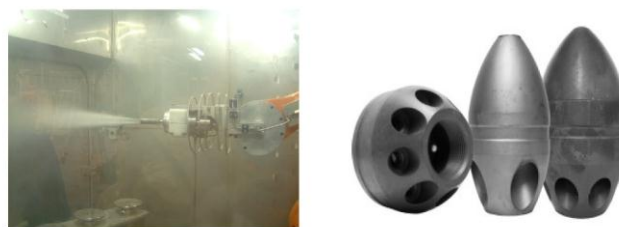
Figure 2 – Flushing Operation and Different Nozzles (Courtesy: Kinloch Equipment & Supply, Inc.)
