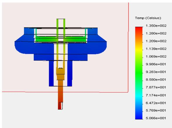
Fig. 3: Temperature distribution of the window assembly obtained from COSMOS (dimensions are depicted in figure 2).
