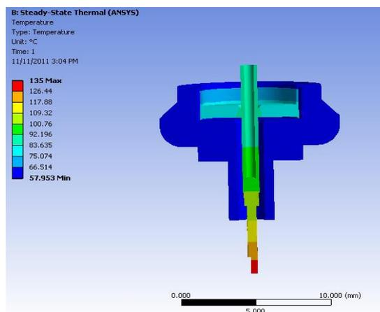
Fig. 2: Temperature distribution of the window assembly for 0.9 mm alumina window disc, obtained from ANSYS (The ratio of outer conductor to inner conductor radii, from top to bottom, are 2.2, 3.5 and 6.1, respectively and corresponding lengths are 9.5 mm, 7.0 mm and 2.0 mm).
