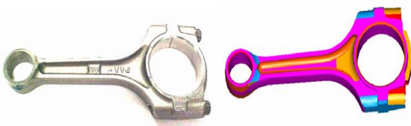
Fig- 3: The actual and the digitized connecting rods.
