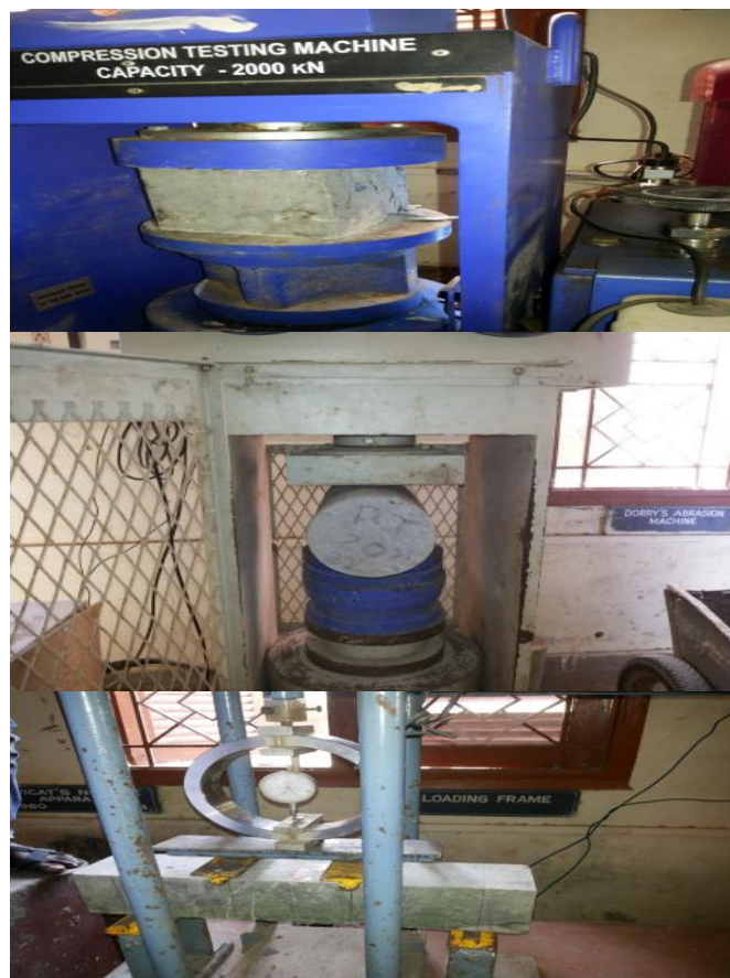
Fig. 3.1 Compression, Split Tensile and Flexural Strength Testing Set ups
