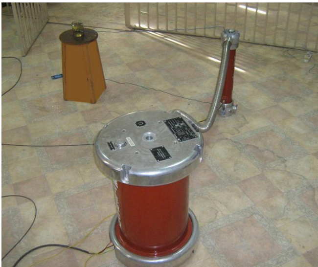
Figure (4): High voltage arrangement for determine break down test
