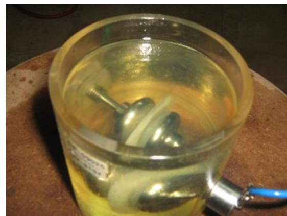
Figure (2): Composite sample which is fitted between mushroom electrode and immersed in oil.
