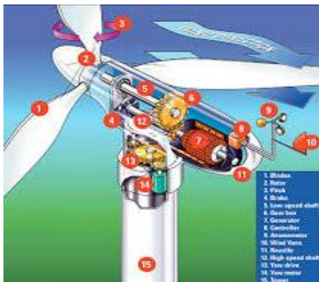
Fig. 6 Wind Power: Wind Mill and its Components [4]
