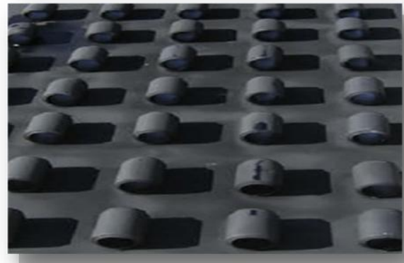
Figure 3: Photograph of Type I arrangement in double solar air heater with aluminium cans
