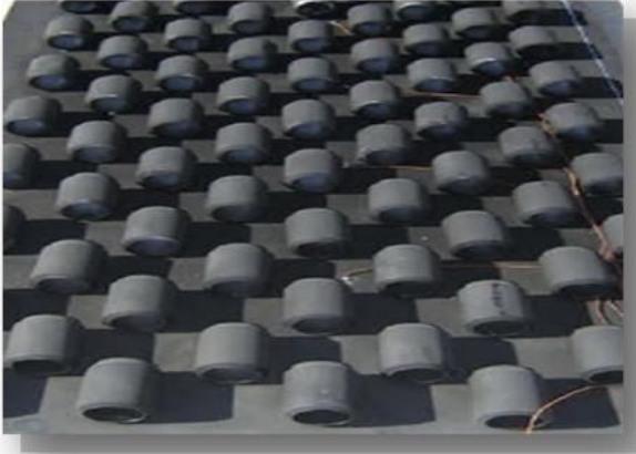
Figure 4: Photograph of Type II arrangement in double solar air heater with aluminium cans
