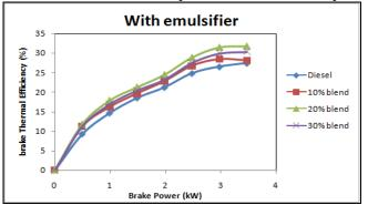
Exhibit 4 Variation of brake thermal efficiency with power output with emulsifier.
