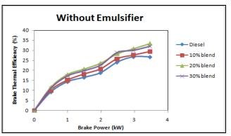
Exhibit 1 Variation of brake thermal efficiency with power output without emulsifier
