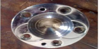
Fig 1: Air gap insulated Aluminum crown (a)Line diagram (b) photo of Aluminum crown
