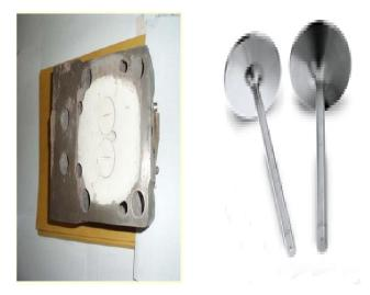
Figure 2: PSZ coated cylinder head and valves
