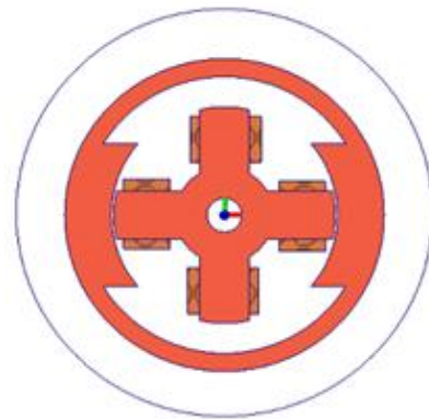
Fig. 1: Conventional 4/2 Exterior rotor two phase SRM
