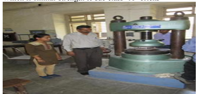
Figure 4: Setup of Compression strength testing machine
