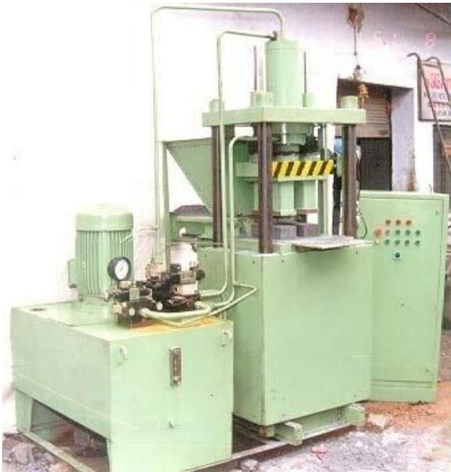
Figure 6 : Double acting hydraulic brick press developed to ensure production of high quality fly ash bricks with application of pressure on both sides and commercialization of C - brick press for production of fly ash bricks have been facilitated.
