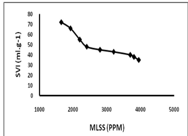
Fig. 16 Change in SVI of sludge as a function of MLSS in the reactor during continuous study
