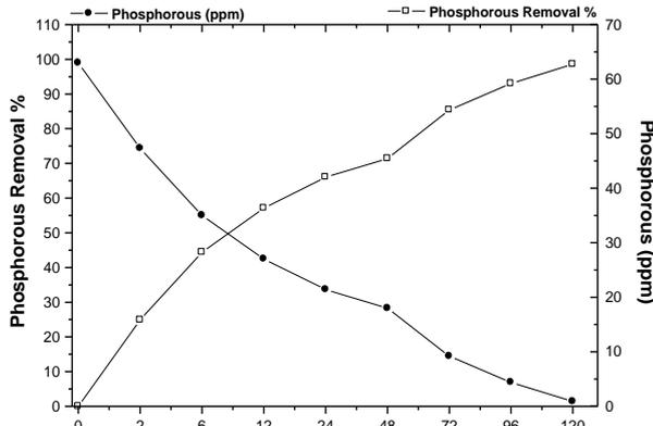
Fig. 11 Effluent phosphorous profile during continuous study
