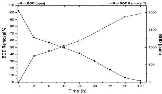
Fig. 5 Effluent BOD profile during continuous study
