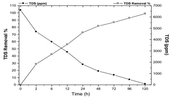
Fig. 9 Effluent TDS profile during continuous study
