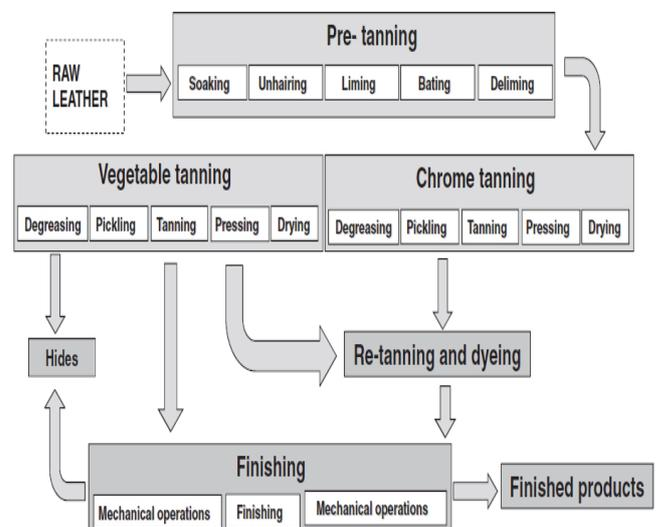
Fig. 1 A typical process flow sheet in an integrated leather tannery industry
