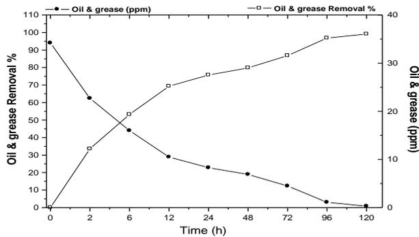
Fig. 12 Effluent Oil & Grease profile during continuous study
