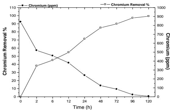
Fig. 13 Effluent chromium ions profile during continuous study
