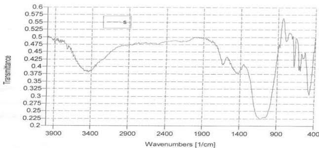
**Fig. 22 FT-IR Spectrum of activated sludge process**
