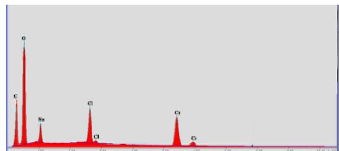
Fig. 20 EDAX analysis of activated sludge process at 24h
