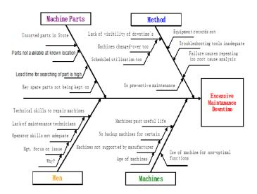
Fig 2. Fishbone Diagram
