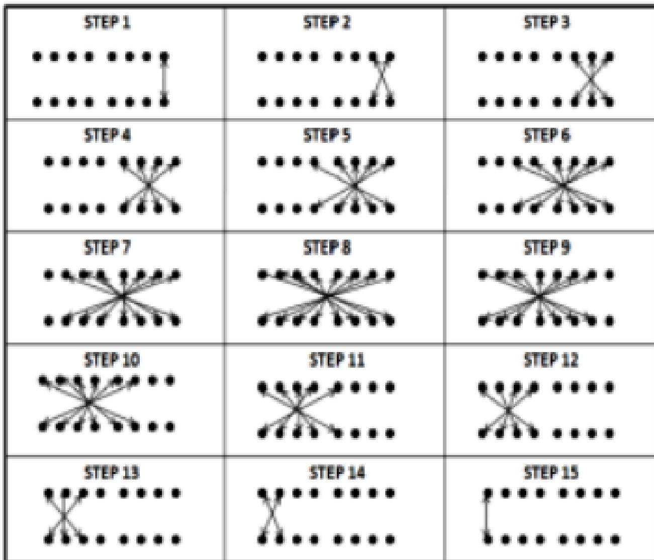
Fig.8-bit binary multiplication using Urdhva Tiryakbhyam Sutra
