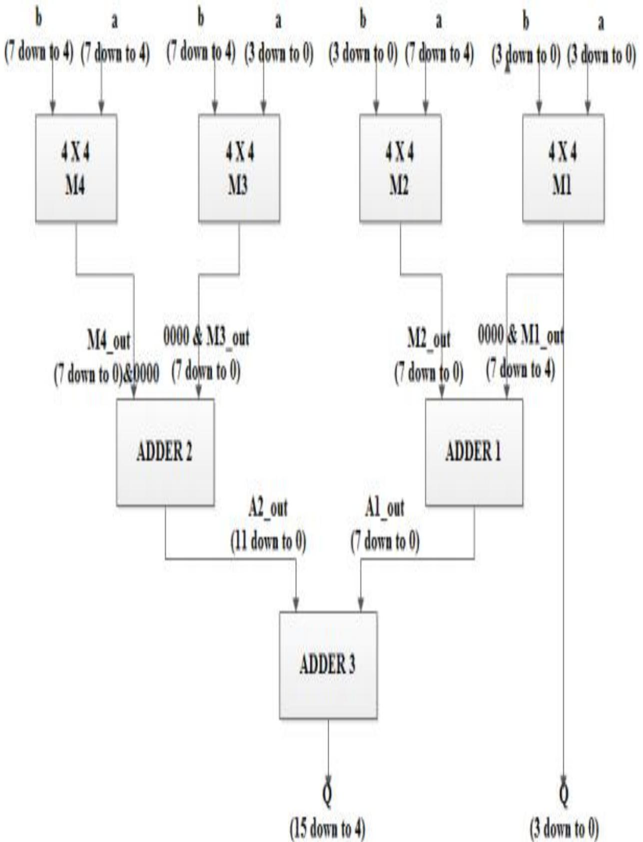
Fig.: Hardware realization of 8 x 8 multiplier
