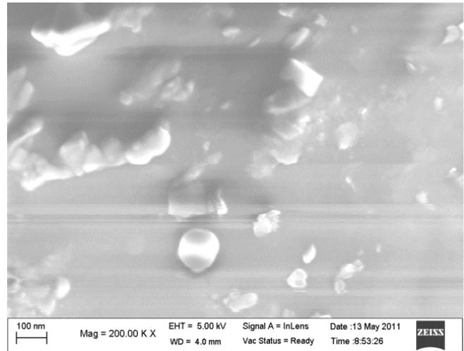
Figure 2 SEM micrographs of 7:3 PMMA/Fe<sub>2</sub>O<sub>3</sub>.
