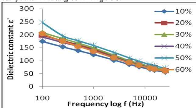
Figure 3. Frequency dependent of dielectric constant ε' at different Fe<sub>2</sub>O<sub>3</sub> Wt%
