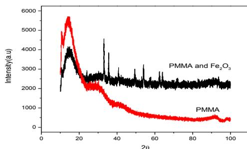
Figure 1. The XRD spectrum of 7:3 Wt% of PMMA/Fe<sub>2</sub>O<sub>3</sub> composite film.
