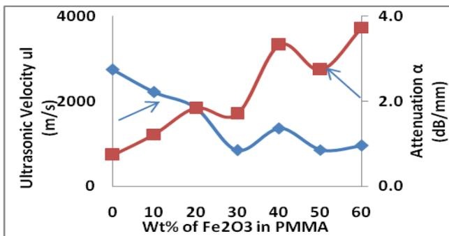
Figure 8: Variation of ultrasonic velocity and attenuation verses against Wt% of Fe<sub>2</sub>O<sub>3</sub> in PMMA
