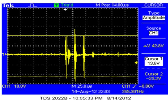
Figure 9: Ultrasonic pulse echo of 70:30 PMMA/Fe<sub>2</sub>O<sub>3</sub> thin film.
