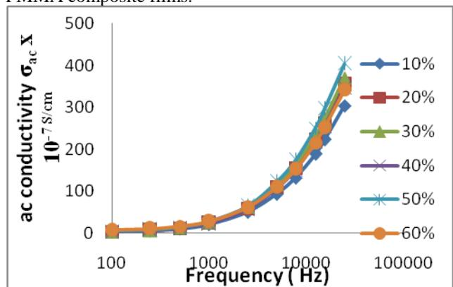
Figure 6. a. c. conductivity as function of wt%. of Fe<sub>2</sub>O<sub>3</sub> in PMMA composites films at different frequencies.
