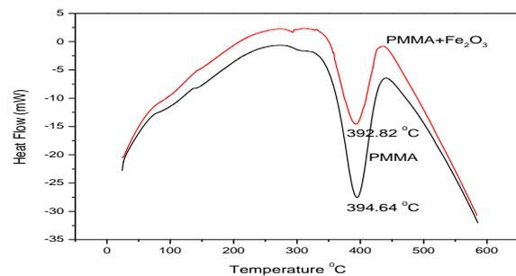
Figure 11 DSC of composite film
