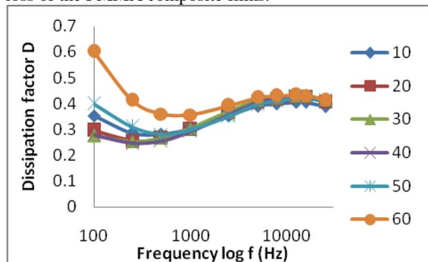
Figure 5 variation of loss tangent of PMMA/ Fe<sub>2</sub>O<sub>3</sub> films at different frequencies
