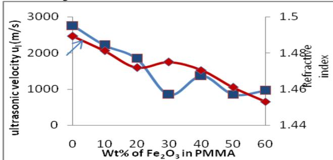
Figure 7: Variation of ultrasonic velocity and refractive index as a function of Wt% of Fe<sub>2</sub>O<sub>3</sub> in PMMA
