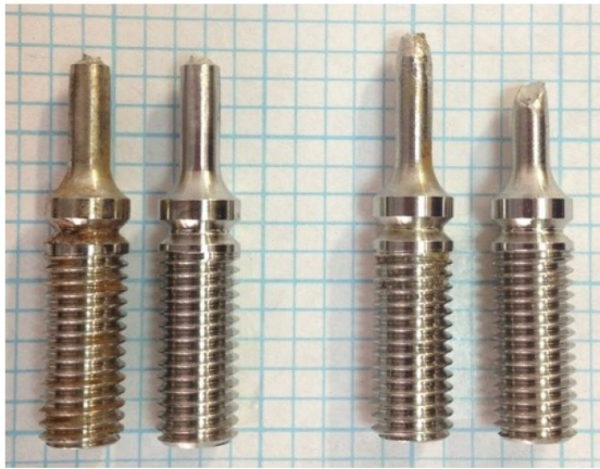
Figure 2. The fractural samples of the notched in ambient, the notched in 5% salt spray, the non-notched in ambient and the non-notched in 5% salt spray from left to right, respectively.
