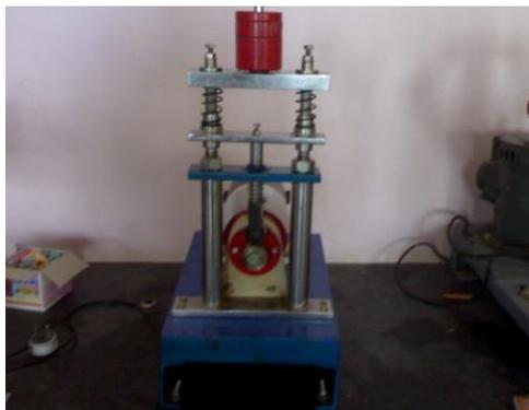
**Fig.2.1 Experimental setup for Analysis of SDOF Vibration**
