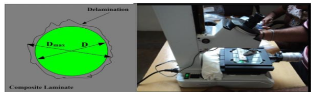
Figure:-8. Schematic view of delamination factor and a view of tool makers' microscope.
