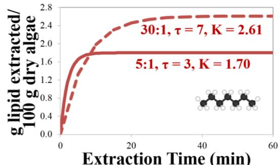
Fig. 14: Comparison of Extraction Kinetics for Heptane at solvent to algae ratios R of 5:1 and 30:1
