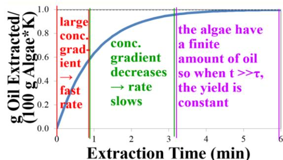
Fig. 5: Example Plot of the Microalgae Lipid Extraction Model.
