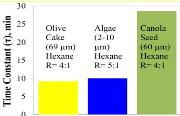
Fig. 18 Hexane Lipid Extraction Time Constant (minutes) for different Biomass Sources, olive cake, *Chlorella vulgaris* microalgae and canola seed
