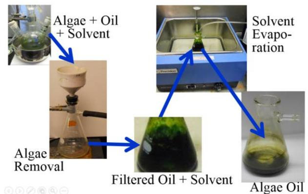
Fig 7: Experimental Setup for the removal of algae and recovery of extracted algae oil from the solvent.
