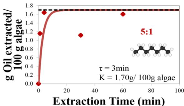
Fig. 11: First Order Extraction Curve for the Heptane solvent extraction of microalgal lipids at a solvent to algae ratio R of 5:1. The computed values of the  $\tau$  and K are shown.
