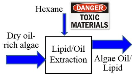
Fig. 4. Schematic of Lipid Extraction from Dry Lipid-Rich Microalgae.
