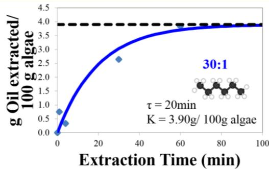
Fig. 10: First Order Extraction Curve for the Hexane solvent extraction of microalgal lipids at a solvent to algae ratio R of 30:1. The computed values of the  $\tau$  and K are shown.
