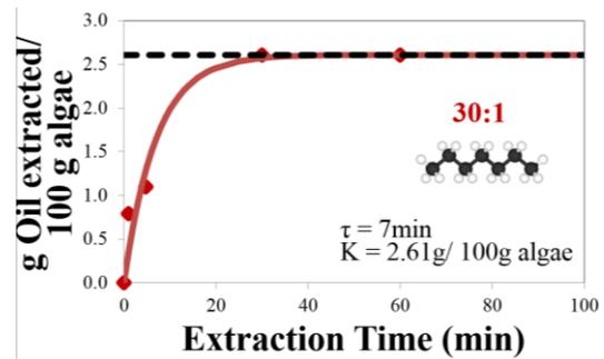
Fig. 12: First Order Extraction Curve for the Heptane solvent extraction of microalgal lipids at a solvent to algae ratio R of 30:1. The computed values of the  $\tau$  and K are shown
