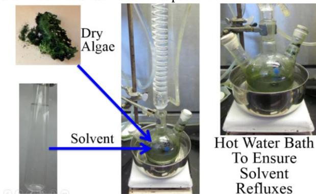
Fig 6: Experimental Setup for the Extraction of Lipids from dry Microalgae using either Hexane or Heptane solvent
