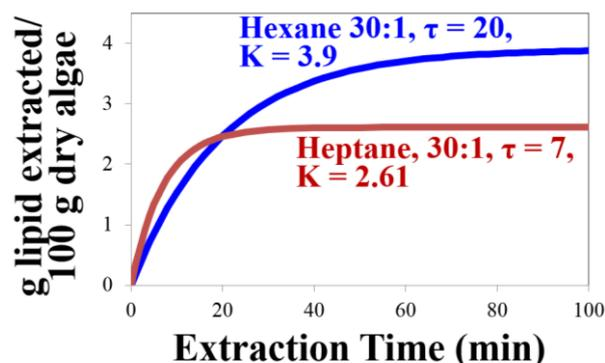
Fig. 17: Comparison of the extraction curves for hexane and heptane at R = 30
