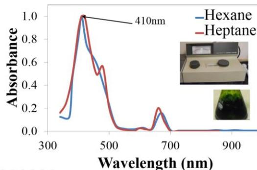
Fig. 8: Spectrophotometer-measured absorbance of extracted microalgae lipids and solvent (Hexane or Heptane) mixture versus Wavelength.
