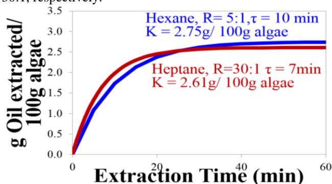
Fig. 15: Comparison of the Extraction Kinetics for Hexane at R = 5:1 and Heptane at R = 30:1
