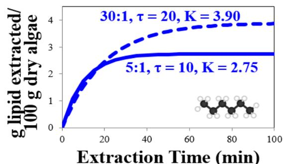
Fig. 13: Comparison of Extraction Kinetics for Hexane at solvent to algae ratios R of 5:1 and 30:1
