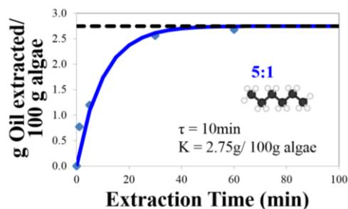
Fig. 9: First Order Extraction Curve for the Hexane solvent extraction of microalgal lipids at a solvent to algae ratio of 5:1. The computed values of the  $\tau$  (minutes) and K (g lipid extracted per 100 g of dry algae) are shown.
