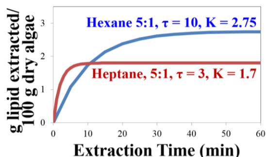
Fig. 16: Comparison of the extraction curves for hexane and heptane at R = 5
