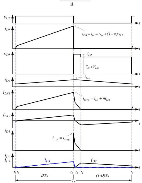
Fig.4. Typical waveforms of the proposed converter at CCM operation.
