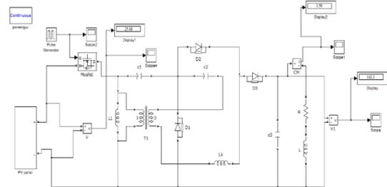
Fig.7.2 Simulink model with RL load
