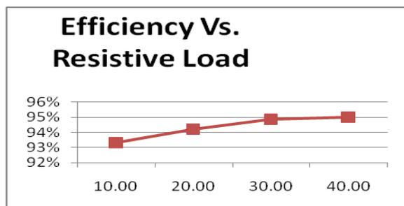
Fig.9 Efficiency versus resistive load.
