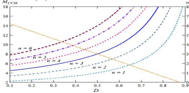
Fig.6. voltage gain  $M_{CCM}$  as function of duty ratio by various turns ratios, and the turns ratio versus duty ratio under voltage conversion is 8.
