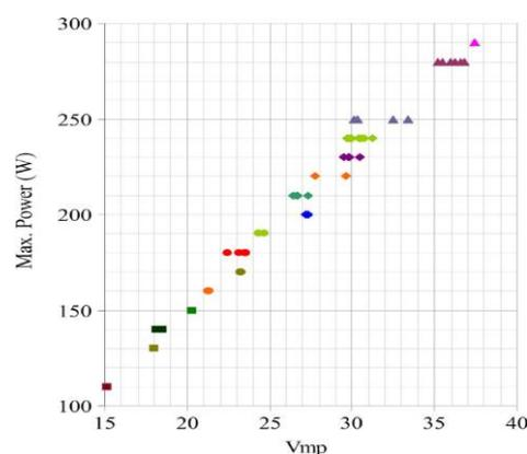
Fig.2 MPP voltage ( $V_{mp}$ ) distribution with various power capacities of PVpanel.
