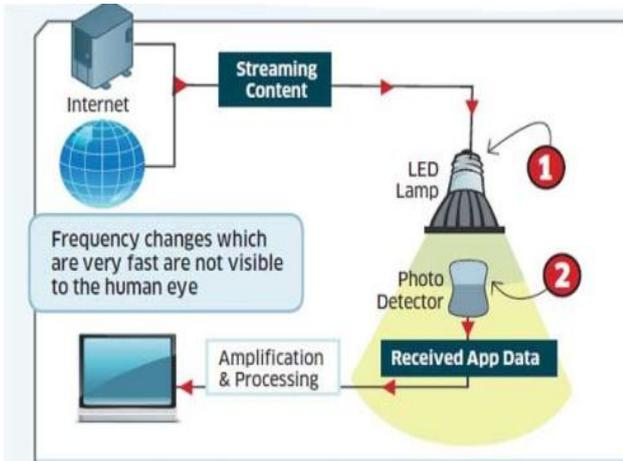
The receiving dongle then converts the changes in the amplitude into an electrical signal which is converted back into data stream and fed into the destination computer or mobile.
