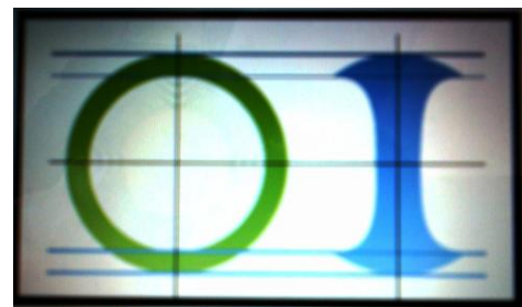
Fig.5 Cross-section of Bamboo and Comparison with an I-Profile
