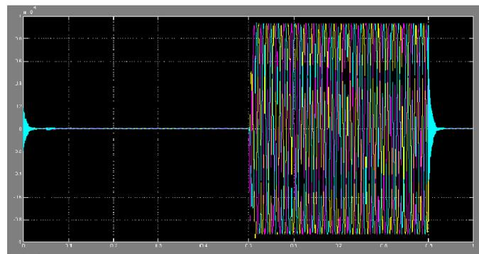
Fig. 9 Simulated output voltage waveform at PCC.
