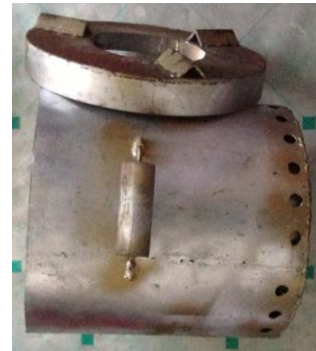
Fig 5: The Side View of the Gasifier Stove
