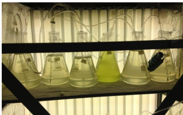
Figure 3. Algae growth in 2 L flasks supplied with air and illuminated with fluorescent lighting.
