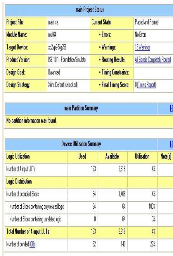
Figure: 4.4 Design Summary of Array Multiplier
