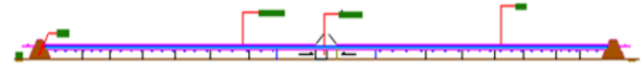
Fig. 4. A tidal power plant 200 m long between training walls following the model of Severn Tidal Power Plant at United Kingdom
