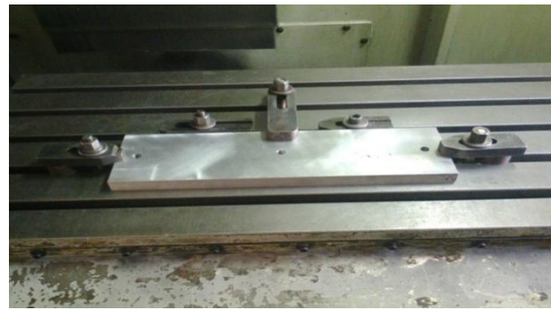
Fig.3 - Workpiece LM 25 plate fixed on m/c table before machining
