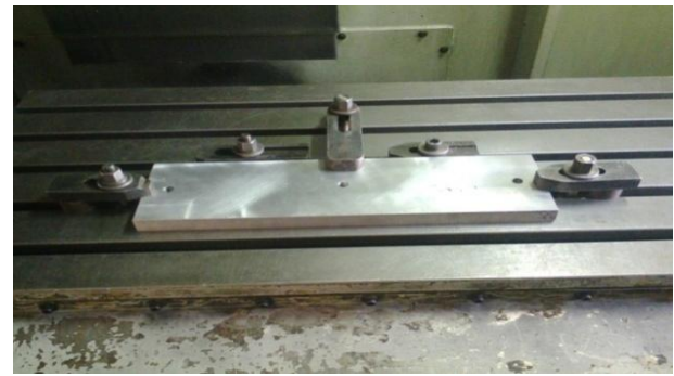
Fig.3 - Workpiece LM 25 plate fixed on m/c table before machining
