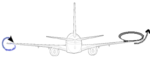
Line drawing of wingtip vortices behind a conventional wingtip (on the left) and an elliptical winglet (on the right)
