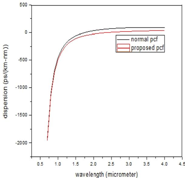
Figure 6 shows the simulated chromatic dispersion of the proposed PCF when  $\Lambda = 2.0 \mu\text{m}$  and  $d = .75 \mu\text{m}$ .
