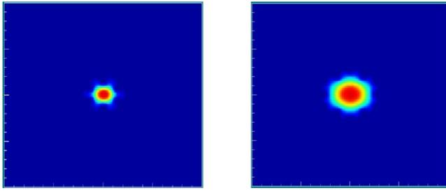
Figure 2 simulated mode field of the (a) normal PCF (b) proposed PCF with  $\Lambda = 2.0 \mu\text{m}$  and  $d = 1.0 \mu\text{m}$  at  $2.4 \mu\text{m}$ .
