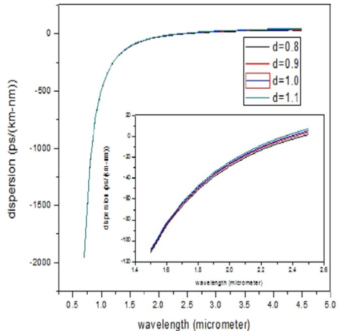
Figure 5 chromatic dispersion of the proposed PCF for different values of the air hole diameter  $d$  when air hole spacing  $\Lambda = 2.0 \mu\text{m}$ .
