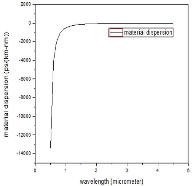
Figure 4. Material dispersion curve of As<sub>2</sub>Se<sub>3</sub> glass PCF.
