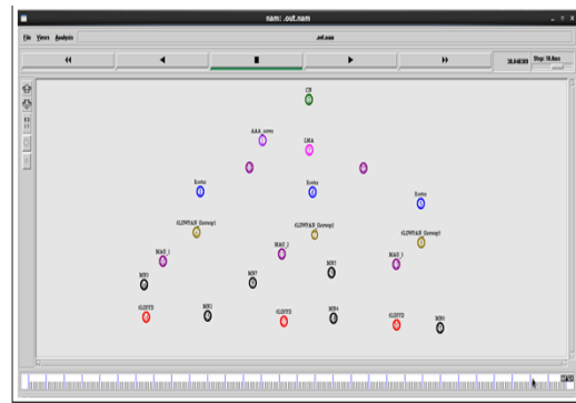
Figure 1.4: 6LoMSN mobility scenario that includes intra-PAN and inter-PAN mobility changes the position of Mobile Node after the simulation
