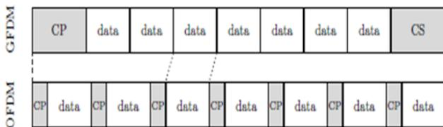
Fig. 5. 2 GFDM and OFDM frame comparison for the MTC scenario.
