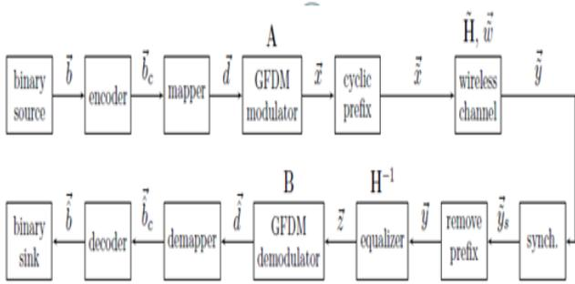
Fig. 3. 1 GFDM Transmitter and Receiver
