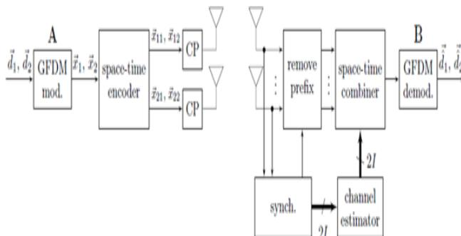
Fig. 4.1 Transceiver block diagram of the STC-GFDM.
