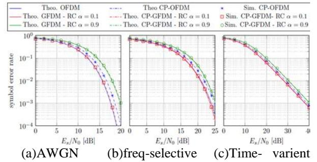
Fig. 5. 3 GFDM and OFDM SER performance in different channel.
