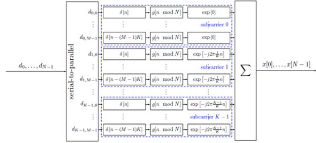
Fig. 3. 2 GFDM Modulator
