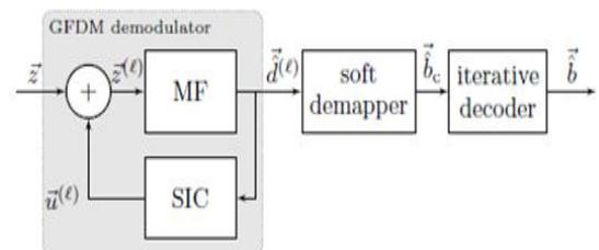
Fig. 4.2(b) MF-SIC Receiver configuration
