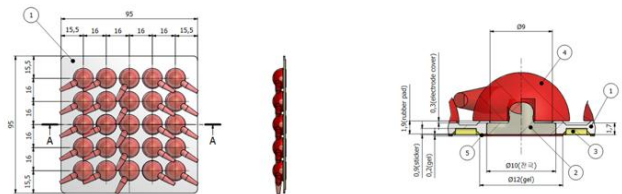
Fig. 3. Probe arrangement and design drawing of MSAE: (a) probe arrangement, (b) designed drawing at the back side of electrode.
