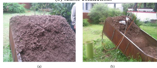
Fig. 5 View of sensor installed at test bed; (a) in-place inclinometer, (b) tiltmeter sensor equations were used for converting sensor's raw data to actual sensor values for the respective sensor. These calibrated equations were incorporated in the landslide prediction software used for continuous monitoring of landslide.
