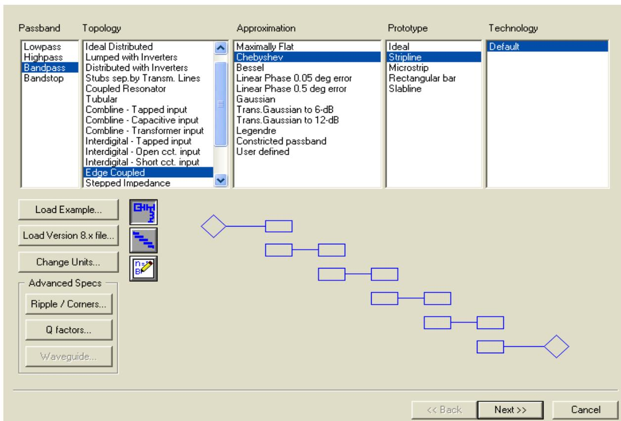
Figure 2 : Working with Filter Design Tool [3]
