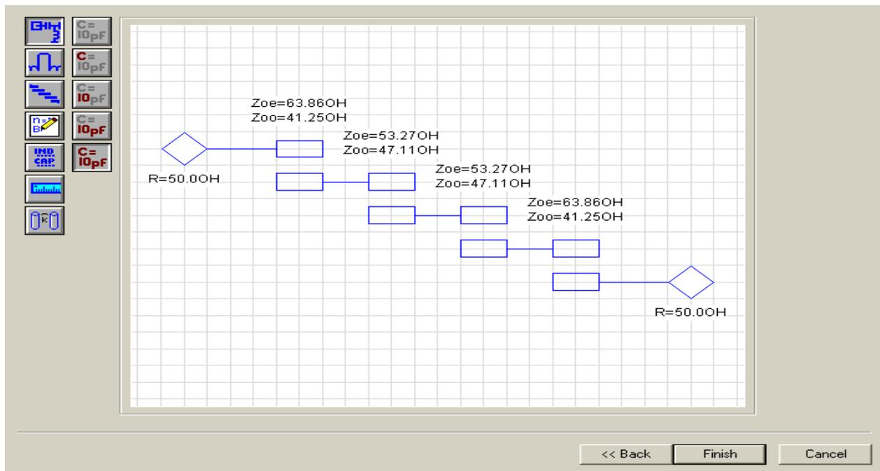
Figure 5: Software Result Of Odd and Even Impedances [3]
