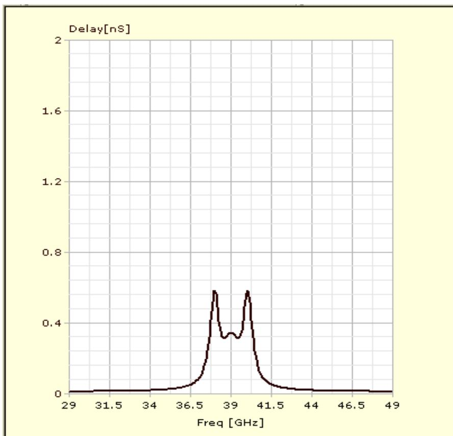
Figure 7 : Simulated group delay result [3]
