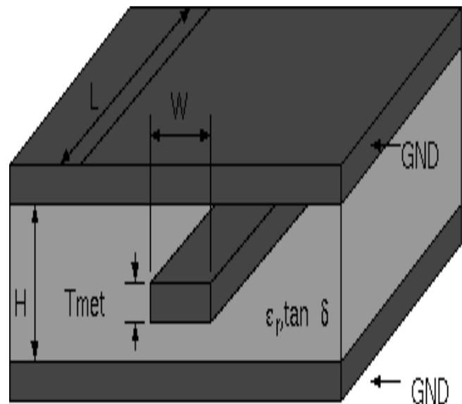
Figure 1: Model used by Designer for edge-coupled Stripline
