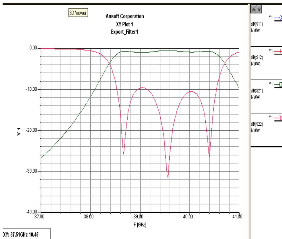
Figure 6 : Simulated Insertion Loss and Return Loss [3]
