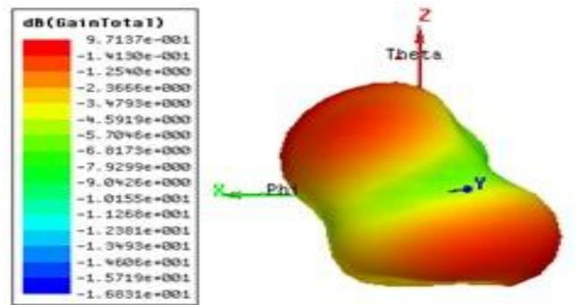
Fig. 5 3D Polar Plot (without shorting pin)
