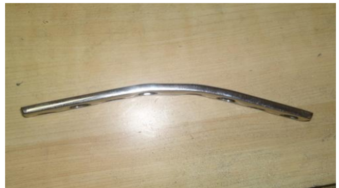
Figure 11The bending plate by mechanical test.
