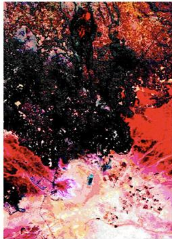
Figure 5 : Color composite of ratio images 3/1, 5/7 and 3/5 prepared Landsat ETM+ expressing the main geological formations.
