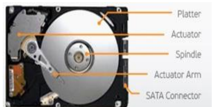
Fig 3.) Platter Based Hard Disk Drive
