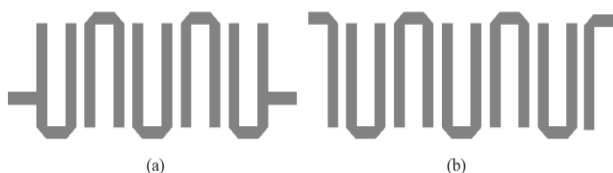
Figure 2.1: (a) tapped line input 5-pole Hairpin Filter (b) coupled line input Hairpin Filter
