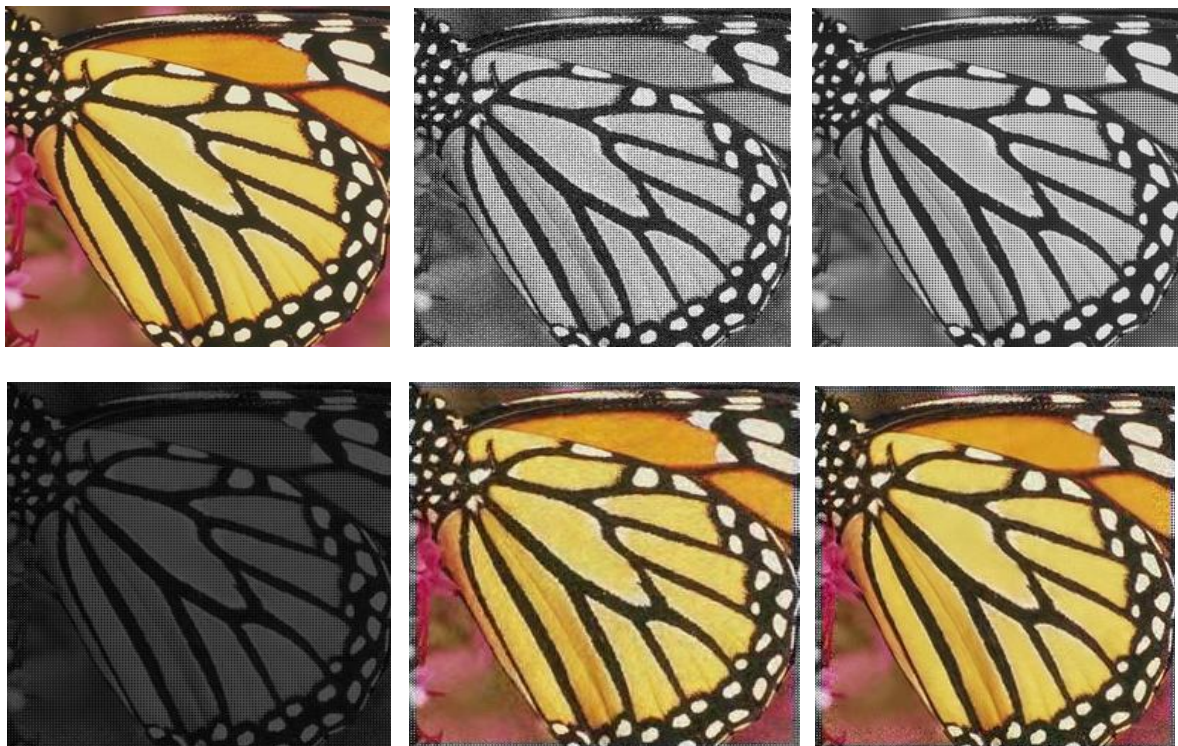
Fig 6. Denoising results of CFA image “Butterfly.” (a) Original CFA image; (b) Noisy CFA image (c) Difference between the denoised and original CFA images by using methods (d) CDM Method (e) Adaptive PCA-based CFA denoising method (f) Proposed Method
