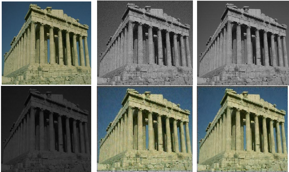
Fig 4. Denoising results of CFA image “ Parthenon ” (a) Original CFA image; (b) Noisy CFA image (c) Difference between the denoised and original CFA images by using methods (d) CDM Method (e) Adaptive PCA-based CFA denoising method (f) Proposed Method
