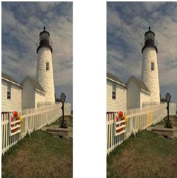
Fig.7. (a) original image(b)Bilinearly interpolated from CFA filter samples with colour artifacts
