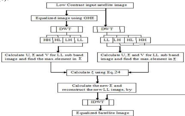
Fig. (c) Detailed steps of the DWT-SVD technique.
