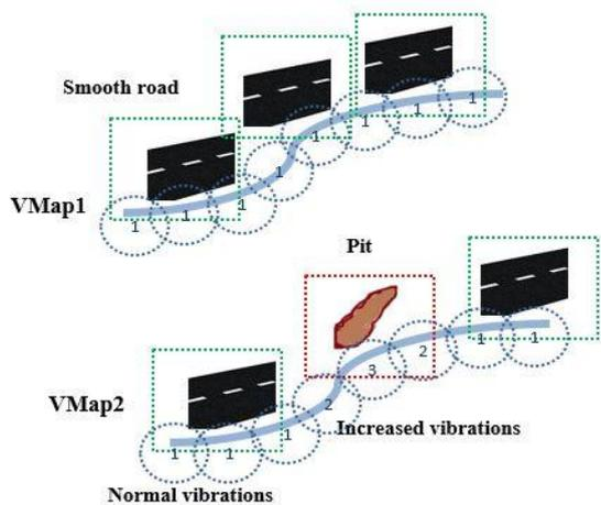
Figure III. Two VMaps showing damage of road
