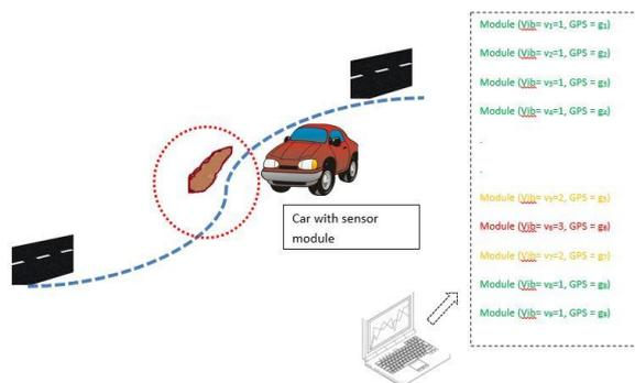
Figure V. System architecture
