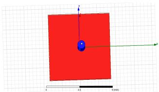
Fig. 2 Microstrip circular patch antenna with shorting pin
