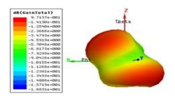
Fig. 5 3D Polar Plot (without shorting pin)
